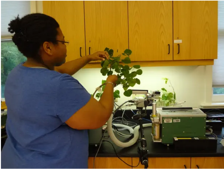
Angelica Patterson uses a photosynthesis machine to measure the rates of respiration and photosynthesis in mature trees. Photograph: Handout
